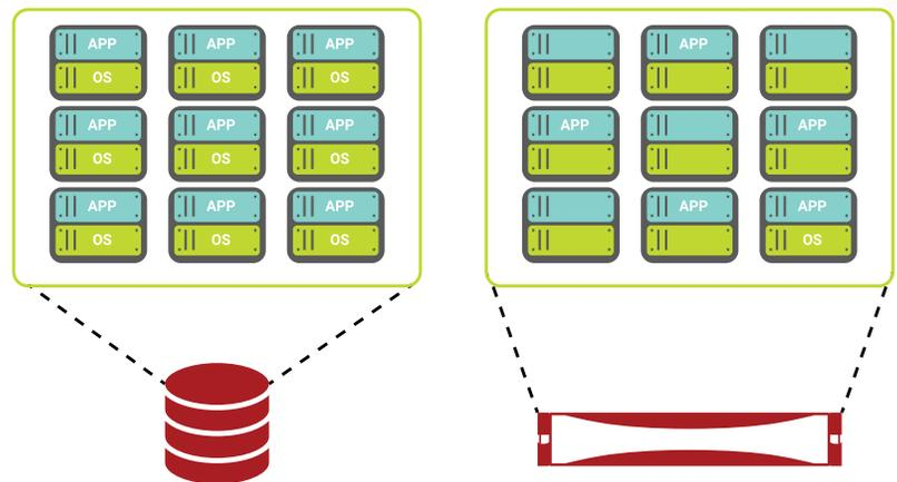
IntelliFlash uses the systems' high-speed storage layers (DRAM, NVDIMM, NVMe, and flash) as a high-performance cache. Data is organized and coalesced prior to landing on the capacity storage layer, turning random I/Os into sequential I/Os. Real-time deduplication then acts as a performance multiplier, freeing up space in the cache for even faster reads and writes. NVDIMMs accelerate cache writes and acknowledgment of I/O leading to extreme performance.
